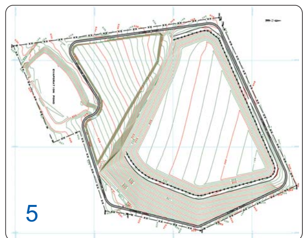
The operational plan is monitored ensuring that predetermined excavation and final height levels are achieved during each phase. This ensures the maximum efficiency in the utilisation of cover materials.
