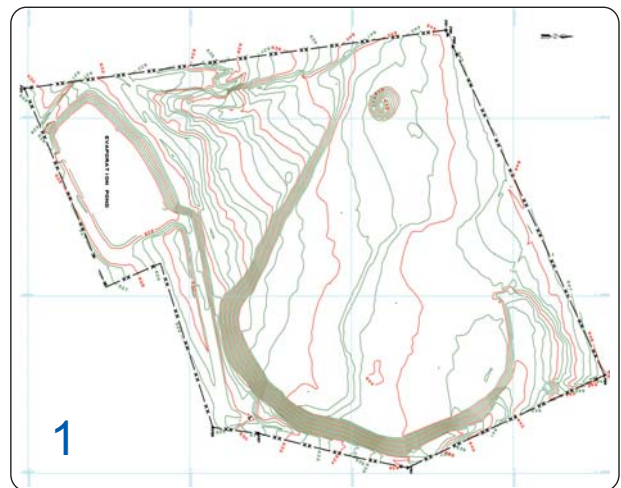
In order to design and compile a future operational plan for a landfill, an accurate survey must be executed and a drawing produced to act as a departure point from which the final model and end-use plan can be determined.
