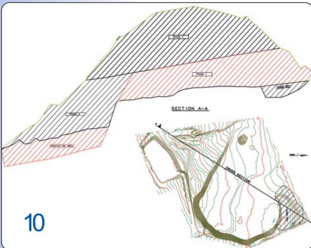
The schematic cross section of the project indicates how the required final profile will be achieved as each phase of operation is systematically implemented.
